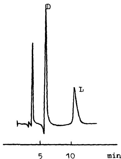
Fig. 3. Separation of enantiomers of \alpha -CF 3 -phenylglycine. Column, Nucleosil Chiral-1, 5 \mu m (250 \times 4 mm I.D.); mobile phase, A-B (75:25), where A = 5 \cdot 10^{-3} M CuSO 4 -10% (v/v) ethanol and B = 5 \cdot 10^{-3} M CuSO 4 (pH 3.0, HCl); flow-rate, 1 ml/min; temperature, 50°C.
